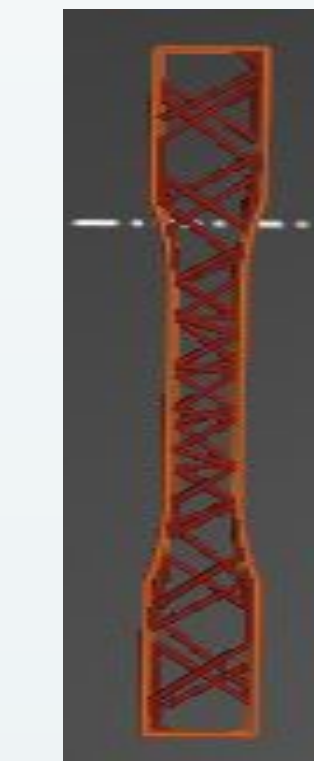
Image of 3D printing model in slicing software where infill can be seen
