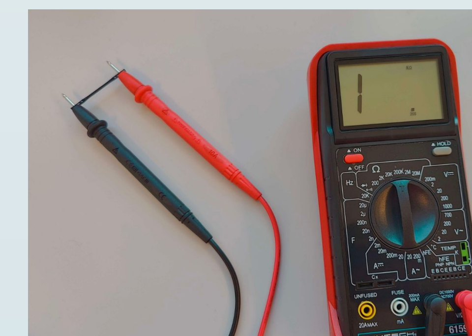
Example setup for the resistance testing of a 3D printed test piece using a multimeter
